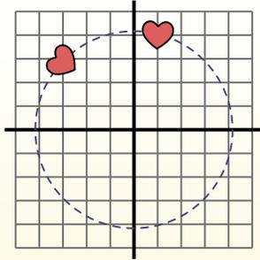
$$1. \begin{aligned} x1 &= 1 \times \cos(60) - 4 \times \sin(60) \\ y1 &= 1 \times \sin(60) + 4 \times \cos(60) \end{aligned}$$
